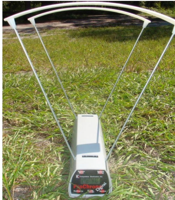
Figure 32 Competition Electronics ProChrono Digital Chronograph
