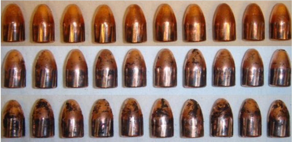
Figure 58 Post-Impact 9mm Bullets, Top to Bottom is Finest to Coarsest
