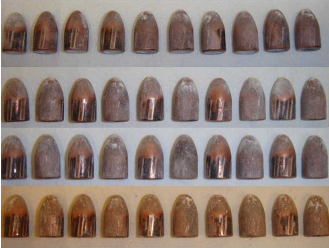
Figure 62 Post-Impact 9mm Bullets, Top to Bottom is Finest to Coarsest
