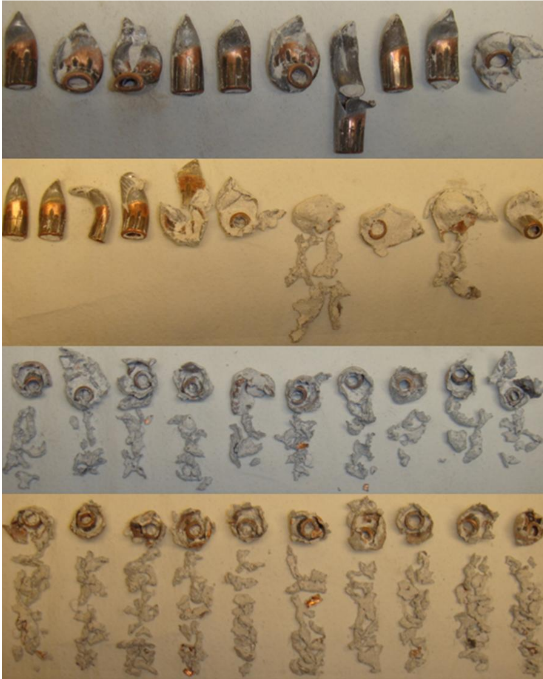
Figure 39 Post-Impact 7.62x39 Bullets, Top to Bottom is Finest to Coarsest
