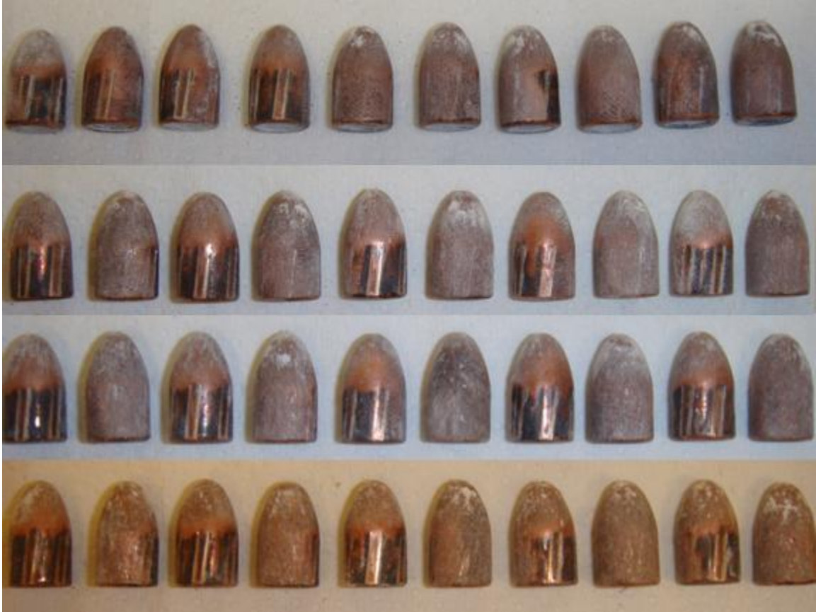
Figure 52 Post-Impact 9mm Bullets, Top to Bottom is Finest to Coarsest
