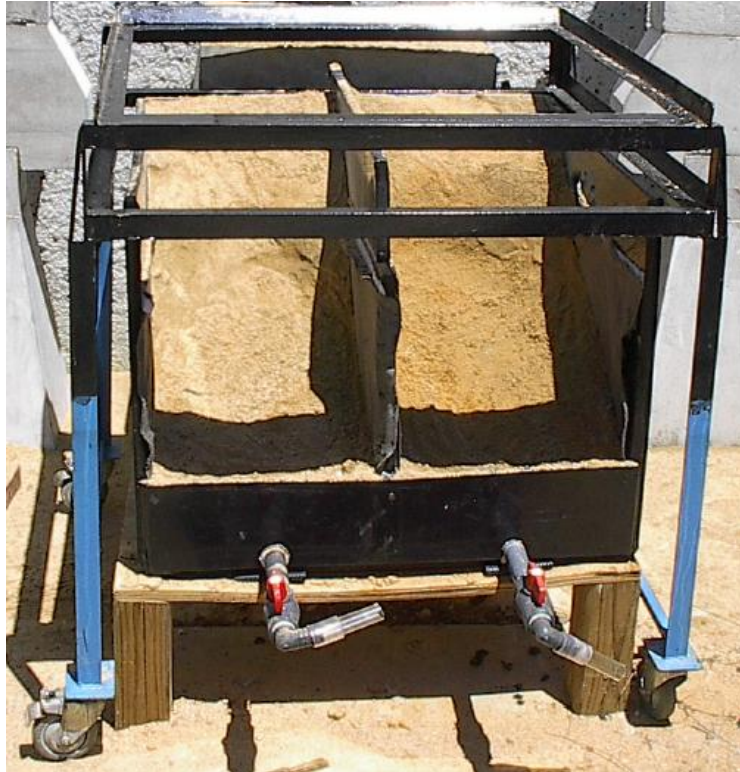
Figure 13 Passive Reactive Sand Berm [3]
