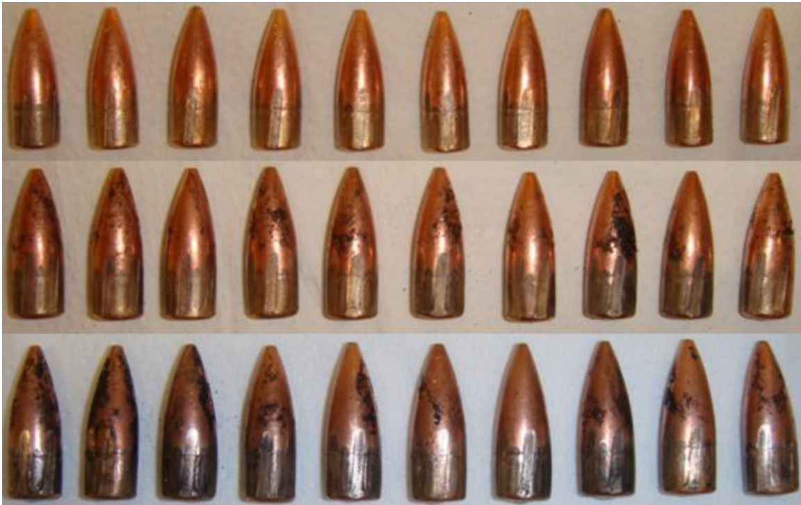
Figure 45 Post-Impact 7.62x39 Bullets, Top to Bottom is Finest to Coarsest
