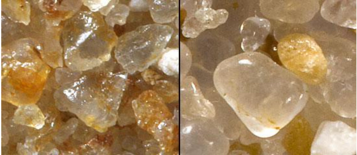
Figure 1 Variation of Roundness and Sphericity of Sand Grains[8]
