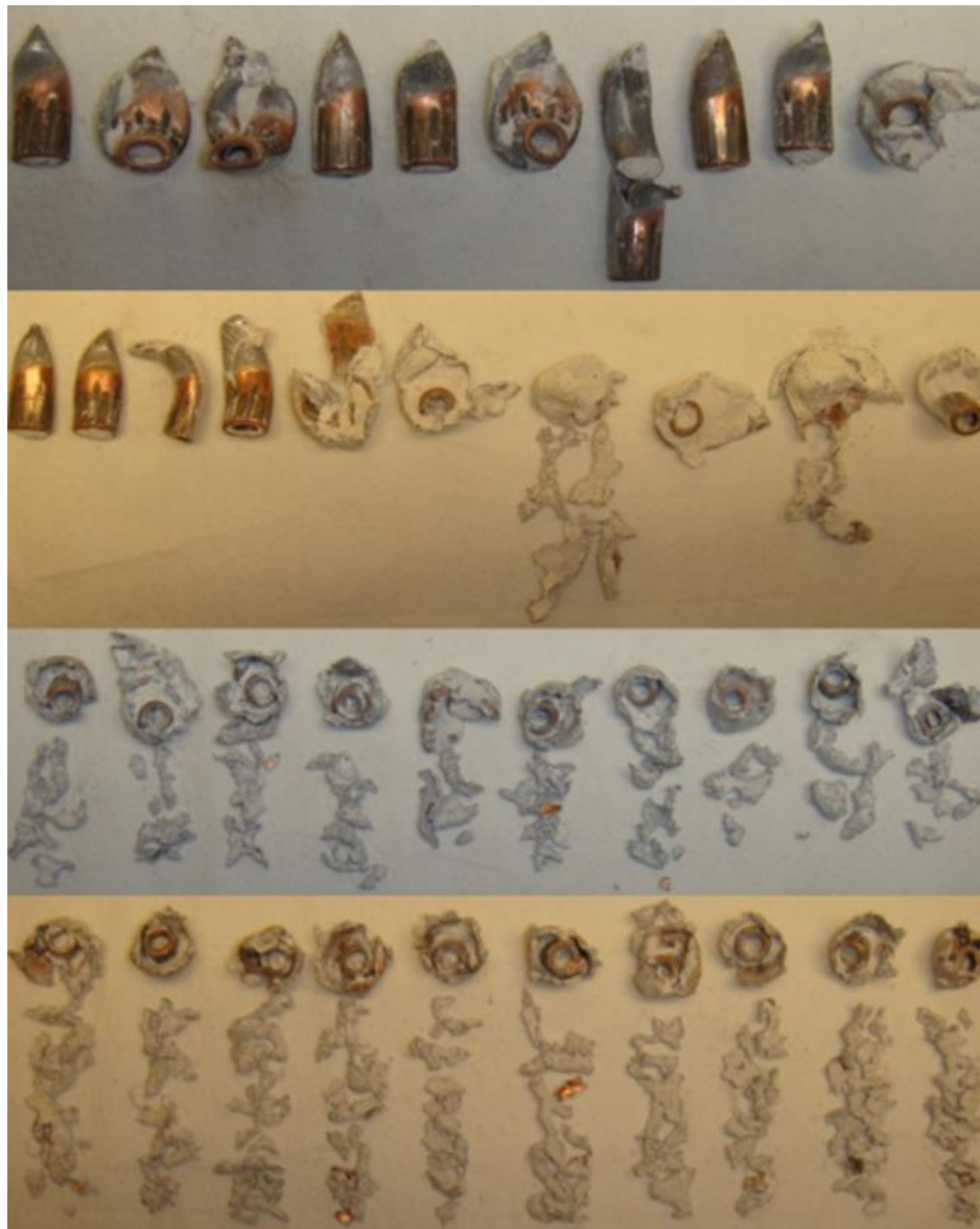
Figure 61 Post-Impact 7.62x39 Bullets, Top to Bottom is Finest to Coarsest
